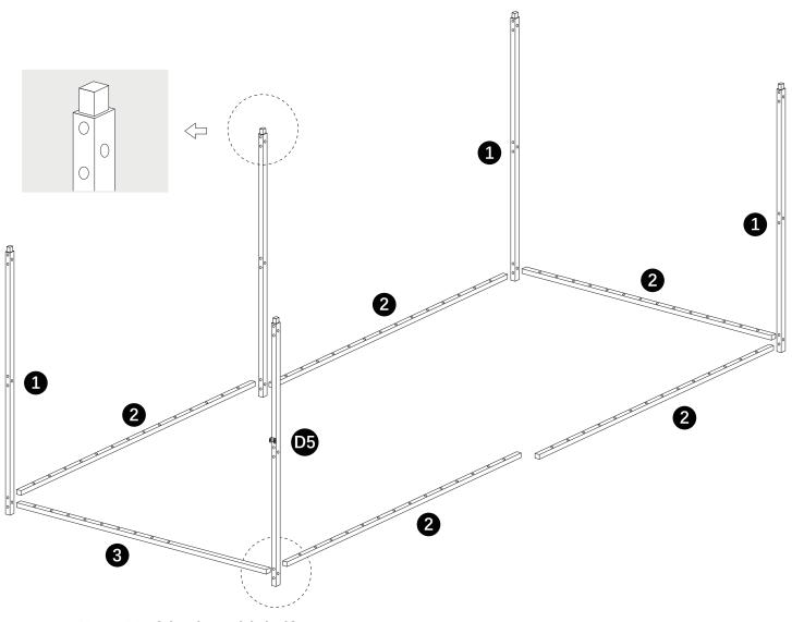
Note: No.3 is pipe with half pre-drilled holes
